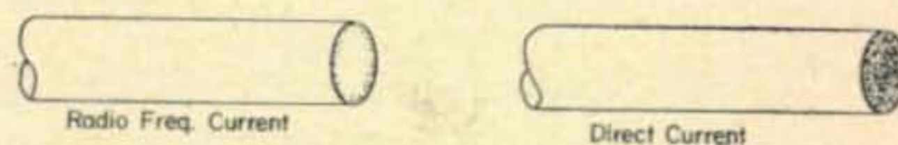
Fig. 5—Cross sectional drawing showing the variation of current density in a conductor carrying radio frequency current. Since the interior of the conductor is surrounded by more flux lines than the exterior, it will have more reactance. As a result there is more current flow near the surface, increasing the effective resistance.
